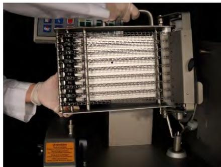
**9.4.11** Replace the chain drive assembly back into its position by lowering it onto its upper guide bin, setting it onto the lower guide pin and the chain drive. Make sure that it is correctly attached to all 3 connection points. Make certain that there are no gaps at connection points and that chain drive is in perfect vertical and horizontal position. Turn upper knurled knob to ensure that chain drive is engaged.
