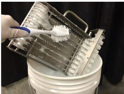
**9.3.6 Use a brush to thoroughly remove all debris in between the rollers and chains of the chain frame assembly.**
