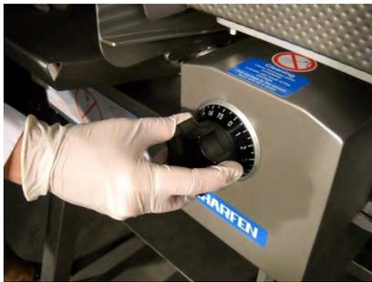
**9.2.1 Close the gauge plate by rotating the thickness adjustment dial, clockwise to zero or as far as possible.**
