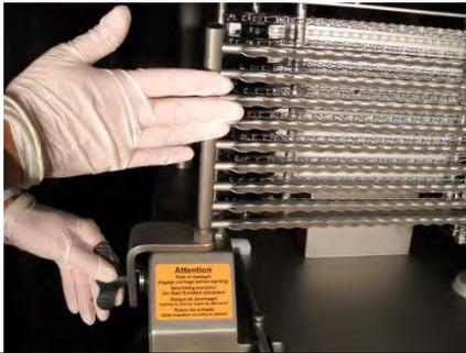
**9.4.12** Attach and securely tighten the stacking arm back into its position and check its correct vertical and horizontal alignment to the chains on the chain drive assembly.
