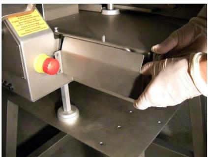
**9.4.14** Attach the side guard by sliding it onto its 2 alignment pins on the machine and securely tighten it into place with the small stainless steel knurled nut.
