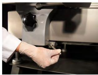
**9.2.16 Disengage the carriage by pushing the locking lever towards the back of the machine.**
