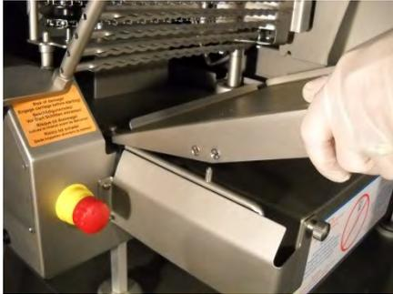
**9.4.15** Replace the stacking table by first sliding it forward onto the rear guide pin and then lowering it onto the guide rod pin.
