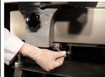
10.4. After the Slicer has been cleaned and reassembled, check that the carriage is disengaged and in "*Cleaning Mode*".
