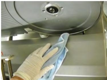
**9.3.3 Clean the carriage, carriage table, thickness plate and the top and sides of the machine with warm water and anti-Bacterial Detergent, the brush and/or cloths. Rinse with clean warm water and wipe dry with clean cloths.**
