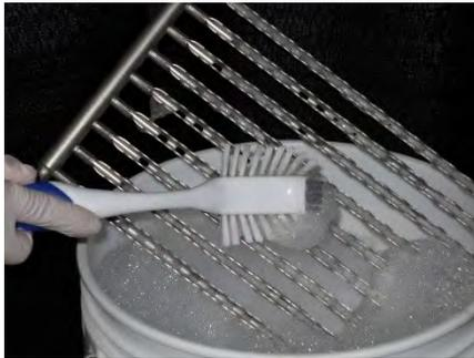
**9.3.5 Clean the stacking arm with warm water and anti-Bacterial Detergent. Use the brush and/or cloths to remove all debris in the stacking arm fingers. Rinse with clean warm water and wipe dry with clean cloths.**
