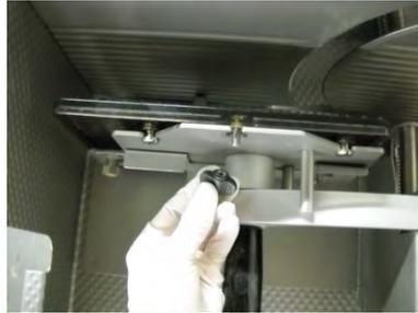
**9.4.8** Attach the food grip plate onto mounting plate and secure into fixed position with round black knob.
